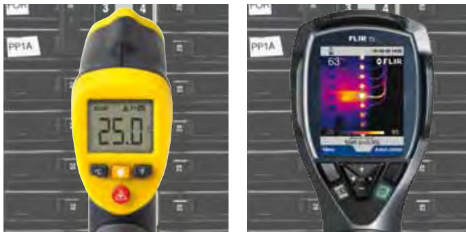
IR thermometer, temperature measurement in one spot FLIR i5, temperature in 6,400 spots
